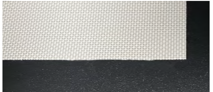
Img. 4 – Fiberglass fray after being trimmed with sharp scissors.
