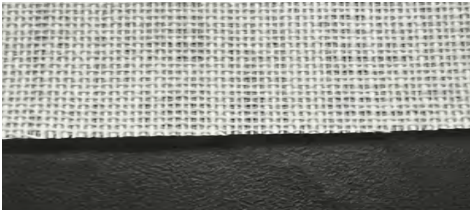
Img. 3 – Polyester fray after being trimmed with sharp scissors.
